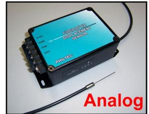
Standard single channel units include amplifier and sensor tip with 914 mm long (3 foot) fiberoptic cable, require +12 VDC input power, and provide 0 to +5 volt analog output with DC - 20 KHz bandwidth.
