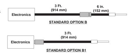
NOTE: Tradeoffs to consider with connectoruzed fiberoptics are reductions in sensor bandwidth capability and slightly elevated noise ripple (2x to 3x higher than normal). The factory should be consulted to determine the suitability of connectorization for demanding applications. We do not recommend more than one in-line connector per sensor system.
