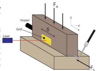
A laser was used to measure local slip,  $\delta$ . Philtec's analog displacement sensor **model D12-H2T4** was used to monitor slip at the top block's leading edge
