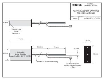
A 19" rack chassis will hold 10 sensor channels. Philtec will deliver five 10-channel racks, each having male & female RS232 serial connectors for daisy-chaining. Distance output on all 50 channels will be read thru one serial port in less than 1 second. 10 channels in one rack can be read thru one serial port in less than 0.2 seconds.
