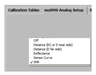
With Option A, muDMS units are provided with two user selectable voltage outputs having a span of 0 to 4.1 volts full scale. These are provided on two BNC connectors. Typically, these outputs are set to provide the Distance Output and the SNR voltage.
