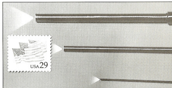
Photo 1. Type 88N sensor tips are provided with fiber bundles as large as 3/16 in. dia. and as small as 0.006 in. dia. Although light rays diverge away from the sensor, they can be reflected back into the sensor tip from an area that is equal to that of the fiber-optic bundle.
