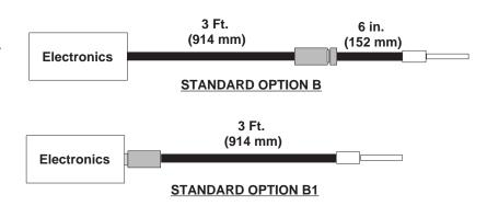
NOTE: Tradeoffs to consider with connectoruzed fiberoptics are reductions in sensor bandwidth capability and slightly elevated noise ripple (2x to 3x higher than normal). The factory should be consulted to determine the suitability of connectorization for demanding applications. We do not recommend more than one in-line connector per sensor system.
