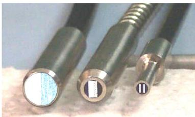
Light is transmitted to the target thru one side of adjacent fiberoptic bundles. The reflected light is captured in two separate fiber bundles which follow independent paths back to the electronics. A ratiometric calculation provides the distance measurement which is independent of target reflectivity variations; i.e., **reflectance compensated**.
