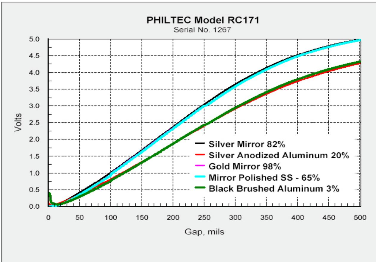
This chart illustrates that reflectance compensation works over a very wide range of target reflectances, nearly 100::1. These data also demonstrate that **reflectance compensation does not correct for the differences between specular and diffuse reflectors**. Specular (smooth and shiny) targets generate about 15% higher sensitivity than diffuse reflective targets...and therefore, different calibrations are required for different surface roughnesses (but not for different materials).
